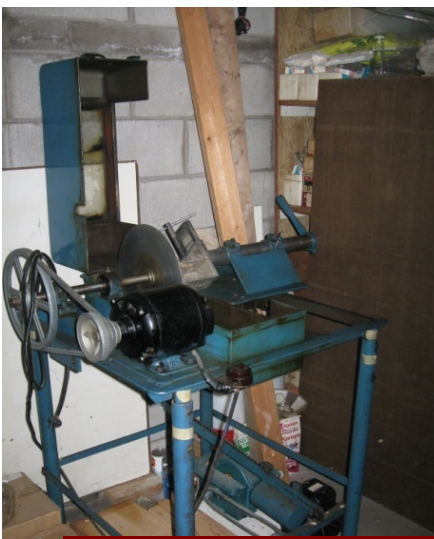
Bill Bingham Designed and Built Lapidary Equipment-Flat Lap With Jam Peg and Saw
