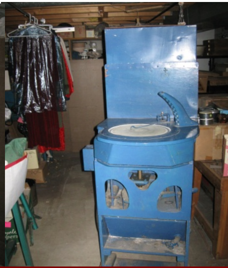
Bill Bingham Designed and Built Lapidary Equipment-Flat Lap With Jam Peg and Saw
