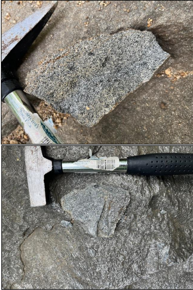
Figure 8 —Examples of Indian Run sedimentary melange in Holmes Run Gorge. Top: A typical Indian Run specimen shows none of the characteristics of schist, such as foliation and a mica sheen. Bottom: A less usual Indian Run rock shows a sheen from tiny muscovite crystals and signs of foliation, such as flaking in parallel sheets.
